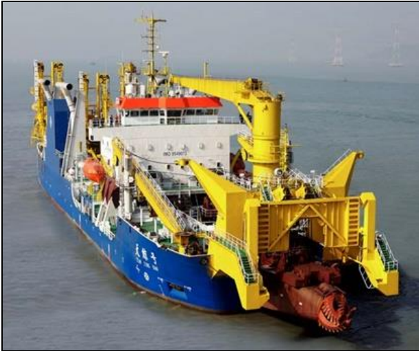
Figure 15: Tian Jing Hao, Cutter-Suction Dredge (Annex 858)
